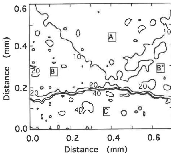
Fig. 5. Contour map of As concentration (ppm) from an SXRfMA area scan over the topaz  $\{110\}$  hillock shown in Fig. 2. Subsector A is below the 10-ppm contour, B and B' are generally within the contours of 10–20 ppm, and most of C is  $>40$  ppm. An oxide inclusion somewhat obscures the A-B' subsector boundary.
