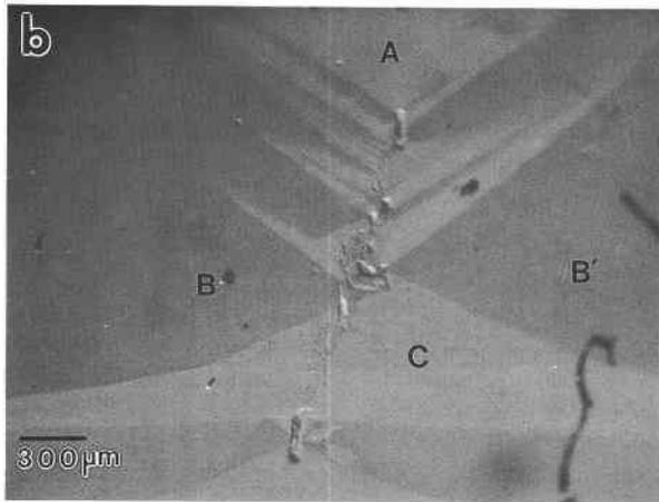
Fig. 3. (a) DIC photomicrograph of a growth hillock on (110) of a second topaz crystal, in the same orientation as Fig. 1. Macrosteps are apparent and show complex growth around an outcropping inclusion. (b) Corresponding CL photomicrograph. Note the strict correspondence of the CL pattern to the complex microtopography and to the mirror symmetry. Observed CL colors are the same as in Fig. 2.
