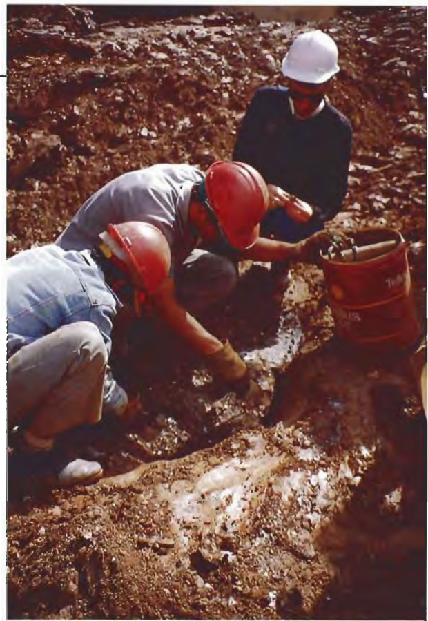
Figure 6. When the bulldozer uncovers a distinctive kaolinite vein, all other activity stops. Certain miners (denoted by red hats) then search for topaz crystals by hand. Here, the senior author examines a topaz crystal found in this thin white vein. Photo by Alice S. Keller.
