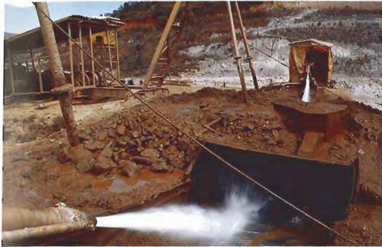
Figure 7. The two drag scrapers bring the host material directly to corresponding platforms at the top of the larger pit, where miners wield large water cannons to wash off the finer particles and push the rock fragments through a series of grates. The largest rocks are screened out first. Photo by Daniel A. Sauer.
